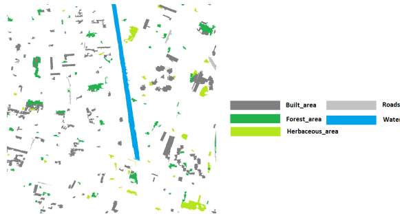
Figure 6: Partial ground-truth map representing urban objects of the VHSR image of Figure 5(a). This map contains 228 segments delivered by a crowd-sourcing campaign in the context of the COCLICO research project. L = 5 different semantic classes are available: built area , forest area , herbaceous area , roads , water .
