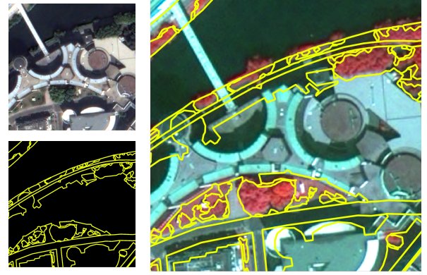
Fig. 2. Misalignment between vectorial topographic data and the actual image. Left: The original image as well as the corresponding vectorial data. Right: False color image with the superimposed vectorial data.
