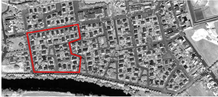
Figure 1: Example of object of interest (an urban block) bounded in red on a panchromatic satellite VHSR image with a spatial resolution of 60 cm (QuickBird, © DigitalGlobe Inc.).
