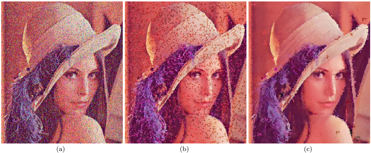
Fig. 8 Filtering results for recursive filtering steps (with different attributes) on lena image affected with salt-and-pepper noise of 50 %. First column: original noisy image. Second column: intermediate denoised image after elimination of compact noise. Third column: final image after removal of compact and elongated noisy structures.
