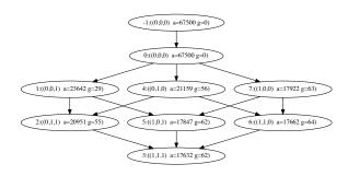
Fig. 7 Component-graph  $\mathcal{G}$  of the segmentation fusion image S. Each node represents a connected component of intersecting segmentations. In each node, the first number represents the node identifier (-1 denotes a fictitious root); then the attributes are: the value of the node, the area of the node and the mean gradient value of the node.
