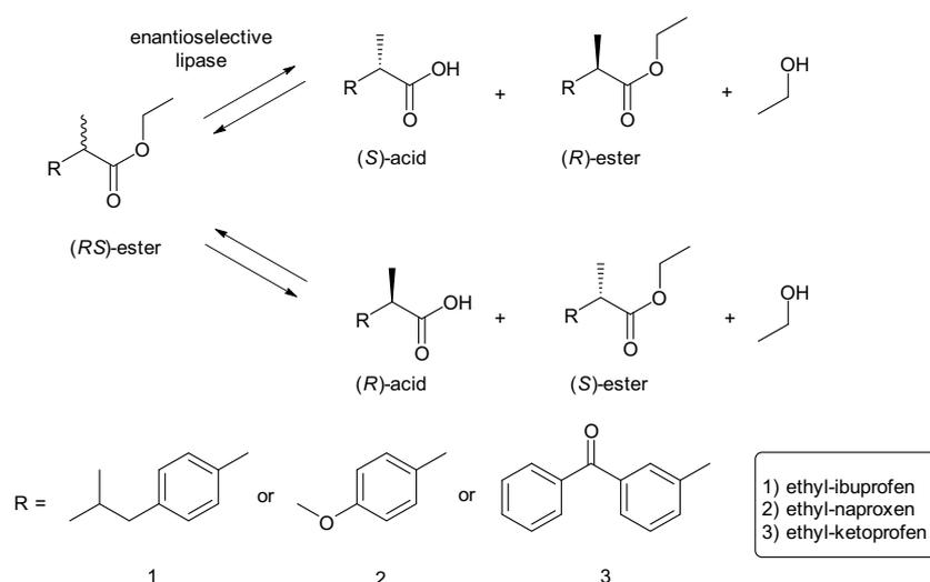
**Figure 1.** Reaction scheme of the lipase-catalyzed resolution of (*RS*)-ethyl ester racemate of ibuprofen, naproxen and ketoprofen by a (*S*)- or (*R*)-enantiomeric lipase (up and down reaction, respectively).
