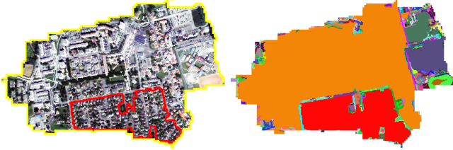
(b) Step 2: extraction of an aggregate of housing blocks (depicted in red).
