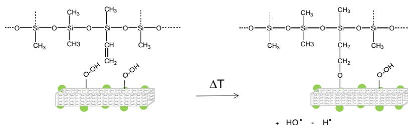
Scheme 3 – Sketch representing the grafting process based on the thermal activation of a peroxidized cellulosic substrate with a silicone matrix including vinylsiloxane units.
