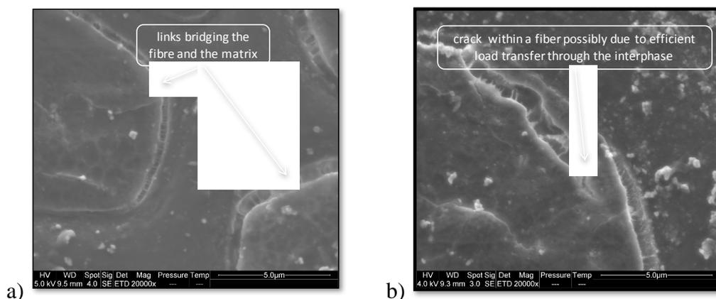
Figure 5 - SEM micrographs of epoxy composites reinforced with flax fabric modified with ELO (16 wt-%) and by EB-irradiation (20 kGy) after tensile testing in the 0° orientation until breakage: (a) surface of matrix zone and (b) cross-cut of the tested specimen.
