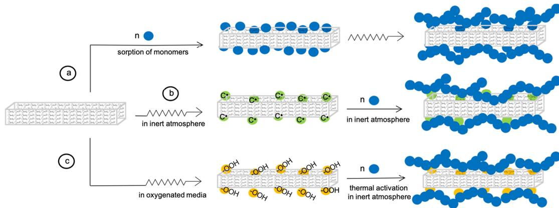
Scheme 1 – Sketch representing the three basic graft polymerization methods using high energy radiation: (a) mutual grafting or simultaneous process, (b) in situ generation of long-lived C-centered free radicals and (c) peroxidation.
