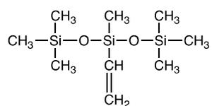
Scheme 4 – Structure of the model vinylsiloxane (1,1,1,2,3,3,3-heptamethyl 2-vinyl trisiloxane) used for grafting experiments onto peroxidized FTA fabric.
