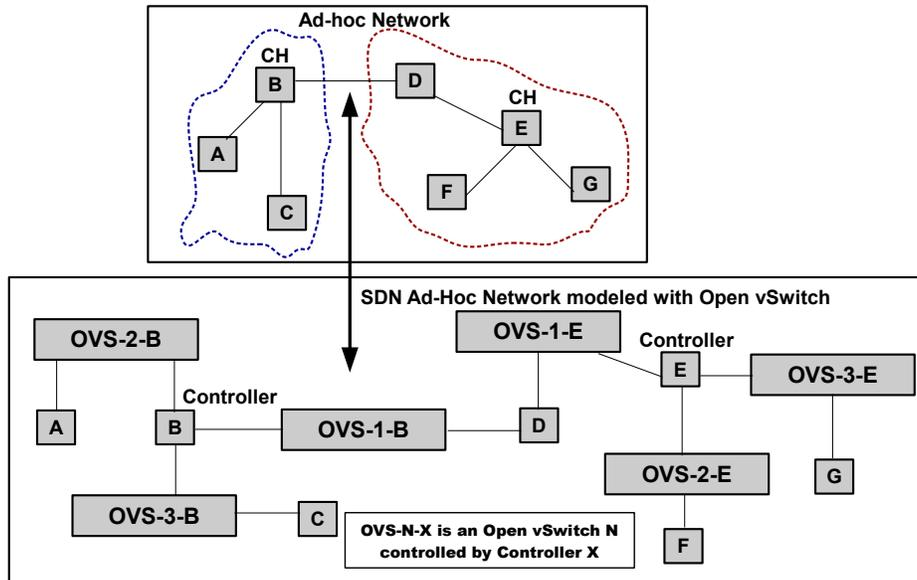
Figure 5. Snapshot of the proposed architecture (SDCSN)
