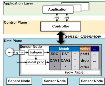
Figure 1. Architecture for Software-defined wireless sensor networks [1]
