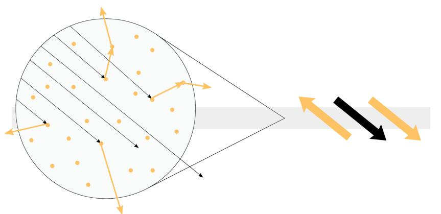
Accounting for the upward and downward directions of propagations in the structure, we thus describe the light distribution at any depth of the structure as a six-flux vector. The net balance relating the total flux sitting on each side of any stack component of the structure (interface, volume layer, or any combination of them) takes a general order-six matrix form.
