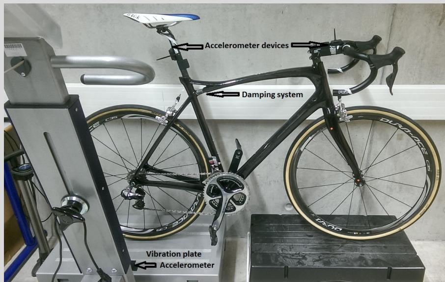
**Figure 1.** Experimental set-up (bike 1, without the cyclist)
