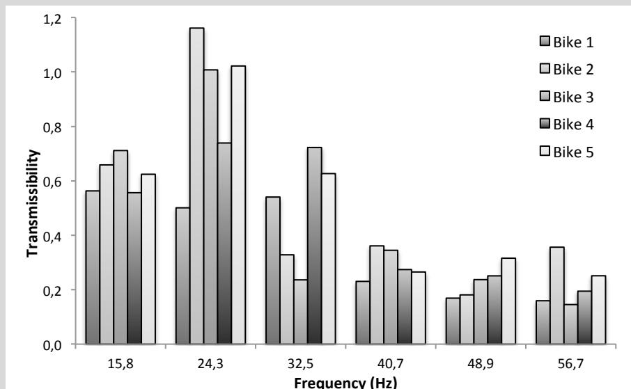
**Figure 2.** Transmissibility stem/platform assessed on the five bike
