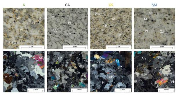
Figure 1: Macroscopic and microscopic photographs (Polarised light optical microscopy) of
