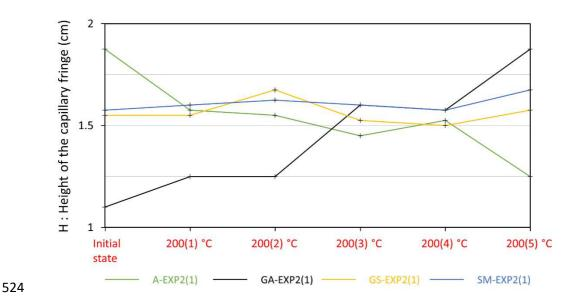
Figure 10: Height of the capillary fringe after the first 10 minutes (H) of capillary absorption
