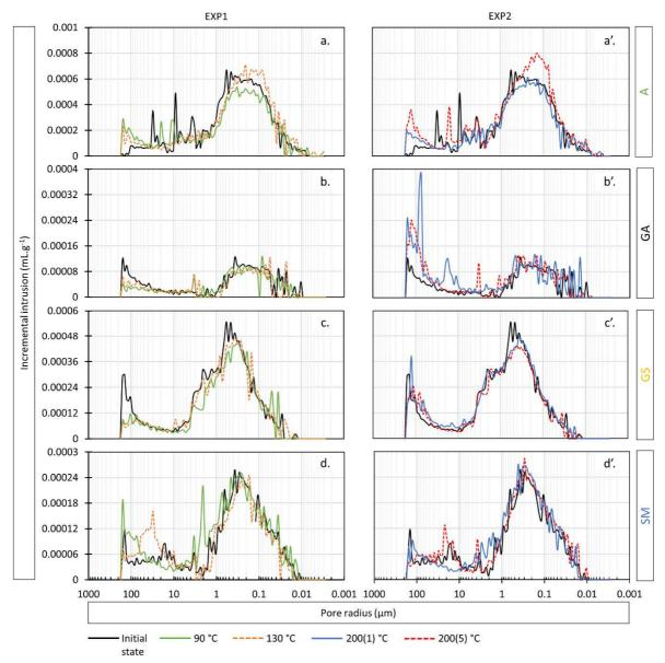
Figure 5: Pore access size distribution curves for EXP1 and EXP2. The curves show the granites tested at room temperature (initial state), 90 °C, 130 °C, 200(1) °C and 200(5) °C. (aa') Albero, (b-b'), Gris Alba, (c-c') Golden Ski, (d-d') Silvestre Moreno.
