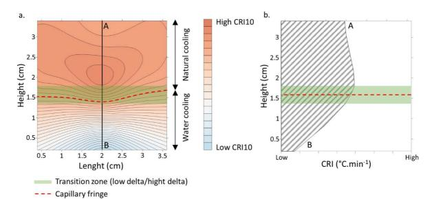
Figure 3: (a) Schematic representation of the cooling rate index (CRI10) on the surface of the samples. (b) CRI10 values along the vertical profile AB. The red dotted line is positioned in the centre of this area. Its position is refined thanks to the isolines on the surface of the sample. Cooling rate index (CRI10) representing the temperature variation per unit of time (10 min).
