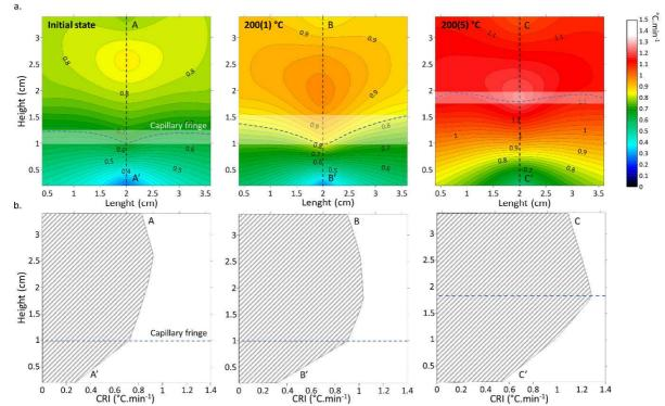
Figure 9: Example of CRI10 mapping (a) and associated profiles (b) obtained by infrared thermography (IRT) monitoring on GA before and after one thermal cycle at 200 °C (200(1) °C) and five thermal cycles (200(5) °C): the dot blue line corresponds to the transition zone and is assumed to correspond to the position of the capillary fringe.
