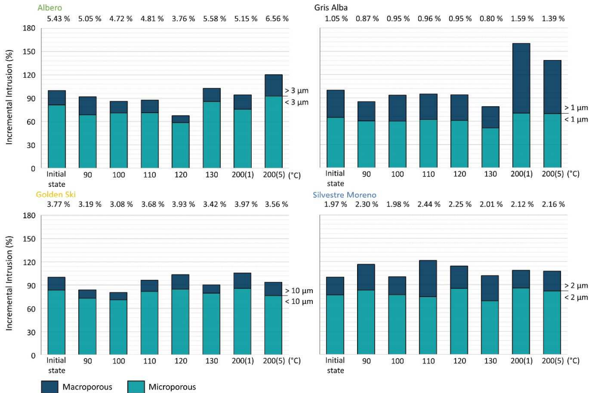
Figure 12: Size distribution of the voids. On the top of each column, the porosity by MIP is detailed.
