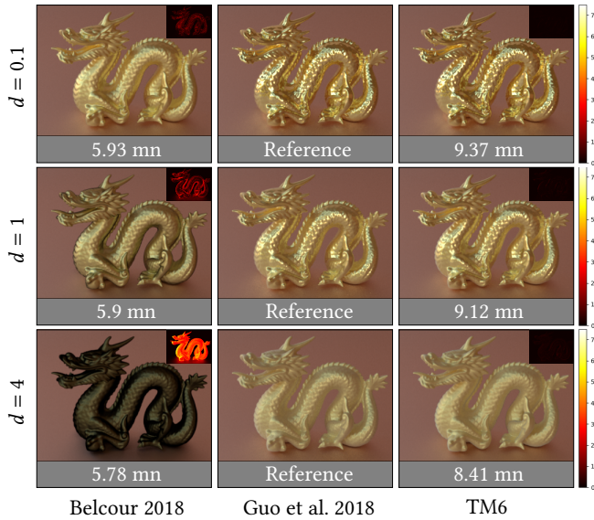
Fig. 15. In the above scene, a non-absorbing scattering medium lies on top of a smooth golden material ( \alpha = 0.02 ). The asymmetry parameter and the scattering cross-section of the medium are respectively set to g = 0.9 and \sigma_s = 0.5 , and the thickness of the volume varies from d = 0.1 to d = 4 . Note how the six-flux approach correctly reproduces the apparent roughness which increases with the thickness of the medium. The results were obtained using 1024 samples per pixel.
