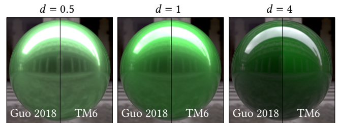
Fig. 21. In the case of scattering dielectric layers, our implementation tends to produce brighter appearances near normal incidences as we do not consider total internal reflections for back-scattered light in the volumes. In the above scenes, a colored scattering dielectric layer with refractive index \eta = 1.5 , scattering cross-section \sigma_s = 0.7 and asymmetry parameter g = 0.9 , lies on top of a conducting base.
