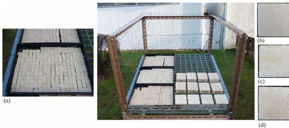
Fig.S1: Platform of stone samples exposure in outdoor. Smaller samples have been collected for the laboratory analyses (zoom of the Courville sample tray (a)) and bigger samples (four for each type of stone) stayed in-situ for the duration of the test for colorimetry and Chl.a fluorescence measurements (zoom of Savonnières sample (b), Ditrupa sample (c), Courville sample (d)).
