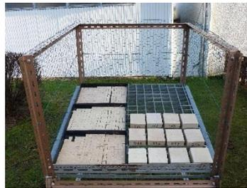
Figure 3. Platform of the biofouling test with samples of different limestones exposed in outdoor. Smaller ones on the left side were collected for IRT testing.
