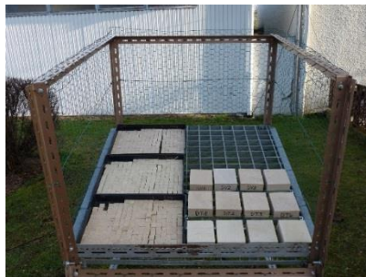
Fig. 6. Platform of stone samples exposure in outdoor. Smaller ones were collected for IRT testing.
