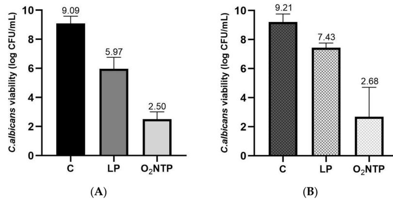
**Figure 2.** Efficacy of non-thermal O<sub>2</sub> plasma on *C. albicans* viability. (A) Contaminated glass slides. (B) Contaminated resin samples. C: Control (untreated samples); LP: 120-min low-pressure exposure; P1: 120-min non-thermal O<sub>2</sub> plasma (O<sub>2</sub> NTP) exposure.
