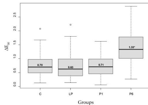
**Figure 5.** Box plots.  $\Delta E_{00}$  of groups C, LP, P1 and P6. P6 showed a significant color change compared to the other groups (C, LP, P1); \* significant difference according to Kruskal-Wallis and Wilcoxon rank sum tests ( $p < 0.05$ ).
