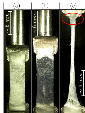
Figure 2: Sample visual aspects for a) dry, b) hydrated and c) hydrated failure states. The red encircled zone highlights the sample failure location.
