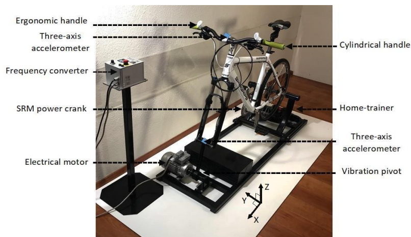
Figure 3: Bespoke cycle ergometer used during the vibration pedalling test and three-axis acceleration measurements.
