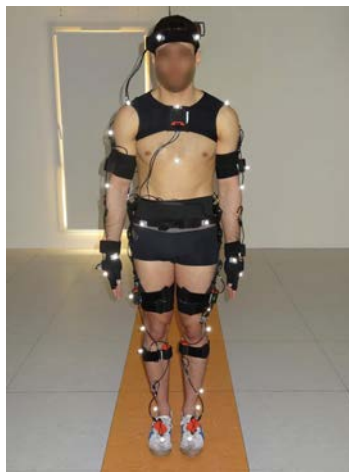
Fig. 1. Quiet stance of a Subject wearing MVN Biomech system and reflective markers of Vicon system.
