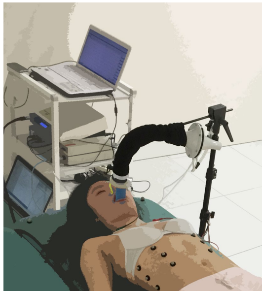
Figure 1. Subject in a supine position with spirometer mounted on a support to limit discomfort and stress.
