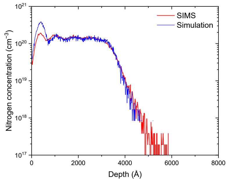
**Figure 3.** SIMS and simulated nitrogen concentration profiles of sample A17. Implantation was realized at 400 °C with a total dose of  $5.4 \times 10^{15} \text{ cm}^{-2}$  and maximal energy of 190 eV.
