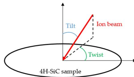
**Figure 1.** Illustration of the ion implantation angles.
