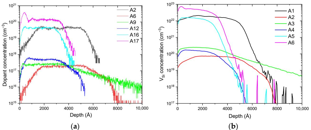
**Figure 4.** Simulated concentration profiles of the dopants (a) and silicon vacancies (b) for samples A2 to A17. All samples are implanted with nitrogen except for A9, which is implanted with aluminum.
