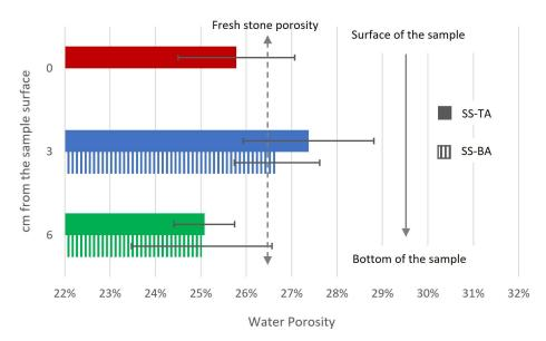
**Figure 4.** Mean and standard deviation of porosity obtained by water absorption. Dark colors correspond to top alveoli samples, and lighter colors to the bottom alveoli samples. The dotted line represents the porosity of the fresh stones. Six samples were used for all the tests except for SS-BA-3, for which only four samples could be prepared.
