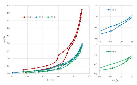
**Figure 5.** Water vapor adsorption isotherms for weathered Crazannes limestone at different depths. SS-0 showed a pore blockage, evidenced by the marked hysteresis. In SS-3 and SS-6, water vapor circulates easily.
