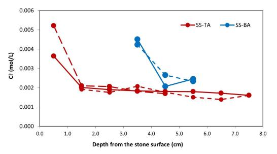
**Figure 9.** Chloride distribution in depth of Crazannes samples. The first analyzed sample had the highest concentration, independently of the position, which is the top (red color, surface at 0.5 cm) or bottom (blue color, surface at 3.5 cm from TA surface) of the alveoli. The second analyzed sample, at approximately 1.5 cm from the surface, revealed lower concentrations that remained stable in depth.
