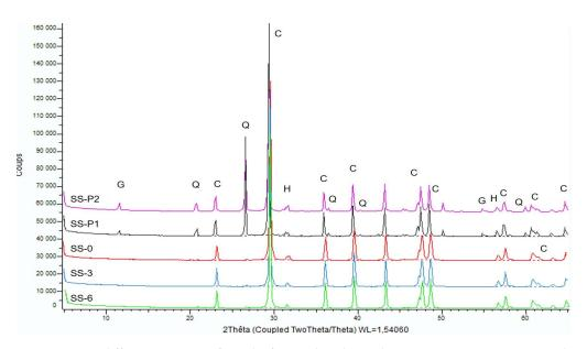
**Figure 7.** X-ray diffraction patterns from the five analyzed samples. G: gypsum; Q: quartz; C: calcite; H: halite.
