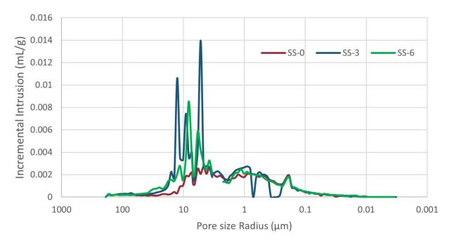
**Figure 6.** Pore size distribution obtained with mercury intrusion porosimetry, showing pore clogging in inner samples.
