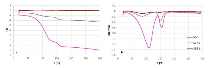
**Figure 8.** (a) TGA and (b) DTA results of powder from alveoli and the surface sample. Gypsum peaks of dehydration are visible on the three samples, although much more pronounced in the alteration products.
