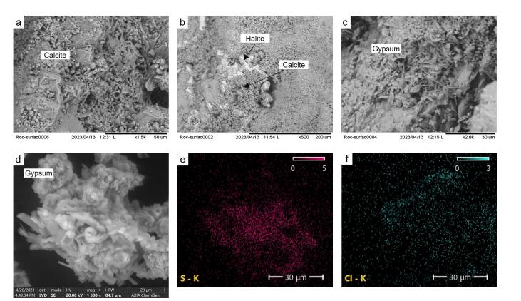
**Figure 10.** SEM images and EDX analysis of samples from the surface and the recovered powder from alveoli. (**a**) Calcite crystals with signs of dissolution and precipitation; (**b**) halite crystals covered by precipitated calcite; (**c**) gypsum crystals on the sample surface; (**d**) gypsum crystal, high resolution image; (**e**) sulfur distribution analyzed by EDX; (**f**) chlorine distribution analyzed by EDX.
