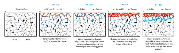
Figure 12. Scheme of salt migration and crystallization with differences in RH (%).
