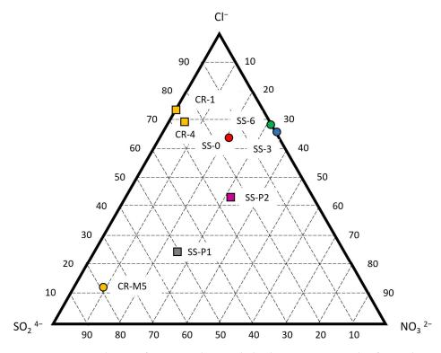
Figure 11. Ternary diagram from IC analysis with the three main anions that form salts.
