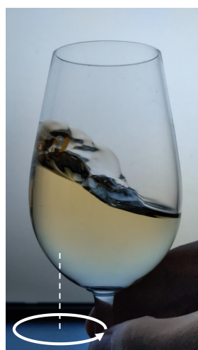
Figure 1. Liquid wave traveling along the sides of a wine glass subsequent to typical manual rotation of the glass conducted with the foot of the glass in full contact with a flat support (desktop).
