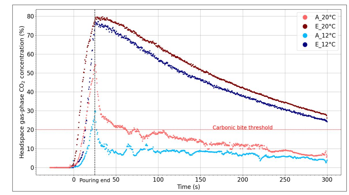
Figure 5: CO<sub>2</sub> concentrations monitoring (in %) in the headspace of **ŒnoXpert** glass (at pixels A and E), during the five minutes following the beginning of pouring 100 mL of champagne. Two different champagne temperatures were examined (i.e., 12 °C and 20 °C)
