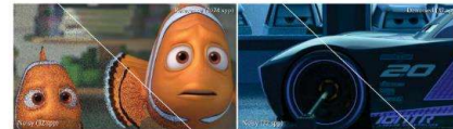
Fig. 1. We introduce a deep learning approach for denoising Monte Carlo-rendered images that produces high-quality results suitable for production. We train a convolutional neural network to learn the complex relationship between noisy and reference data across a large set of frames with varying distributed effects from the film Finding Dory (left). The trained network can then be applied to denoise new images from other films with significantly different style and content, such as Car: The Hub (right), with production quality results.
