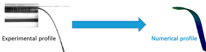
Figure 11. Modeling of yarn by a homogeneous transverse isotropic material.
