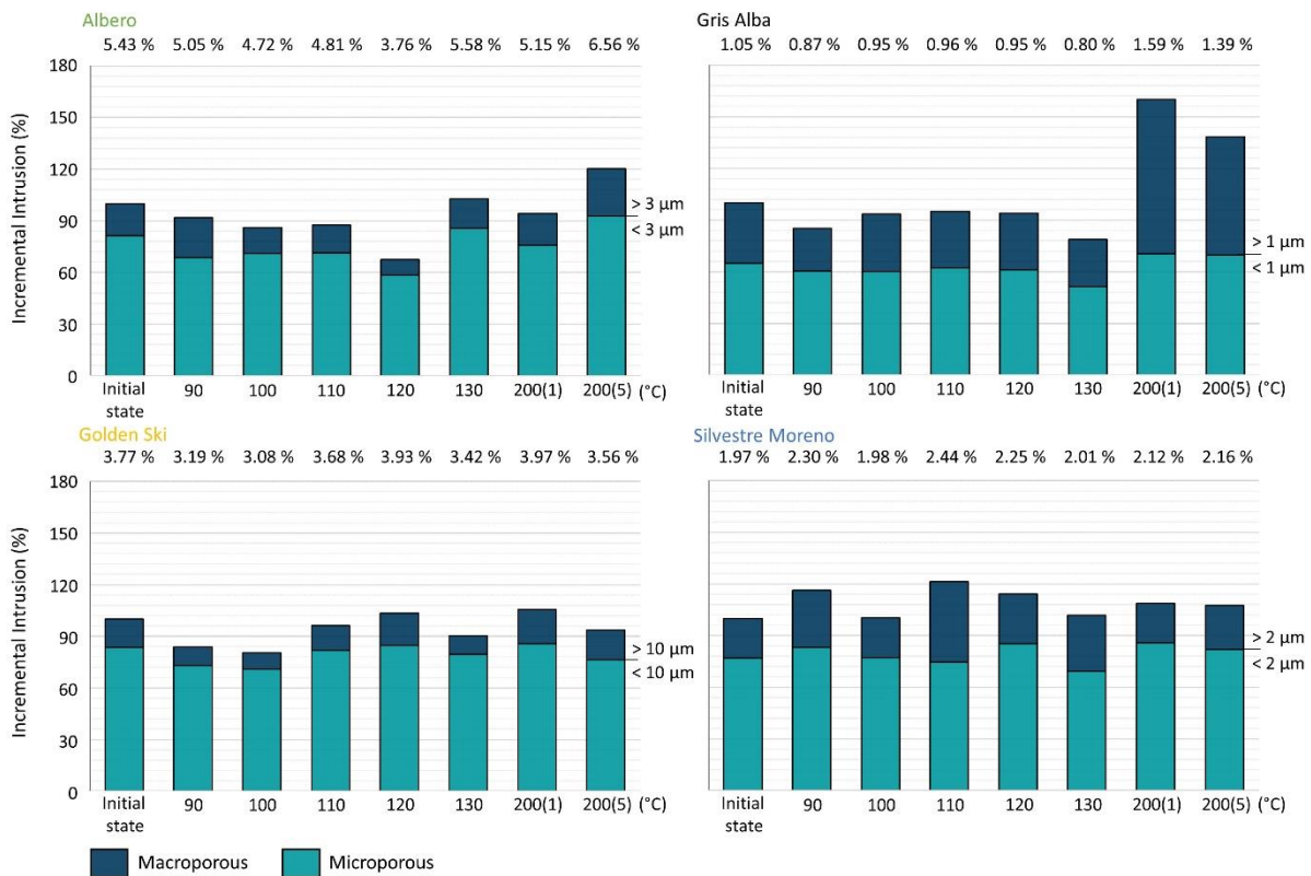
Figure IV-13. Size distribution of the voids. On the top of each column, the porosity by MIP is detailed.
